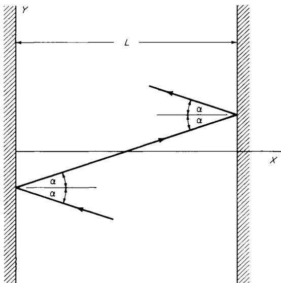
FIG. 33.2. Propagation between two mirrors.
