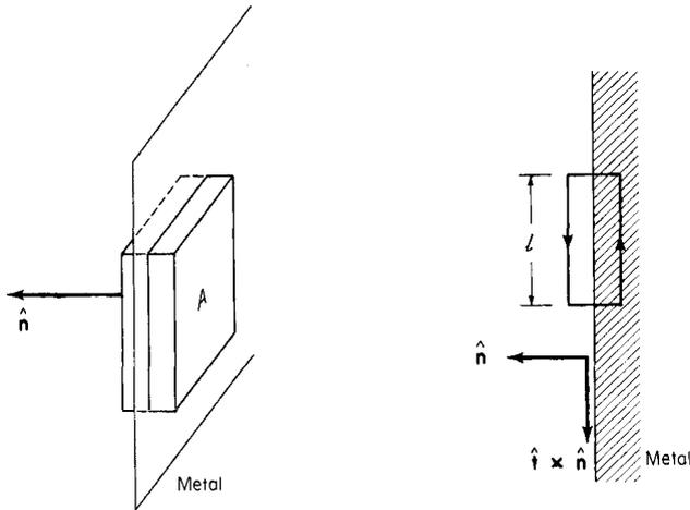
FIG. 33.1. Geometry for obtaining boundary conditions from Maxwell's equations. Here  $\hat{n}$  is the unit normal out of the metal and  $\hat{t}$  is a unit tangential vector.
