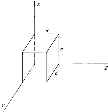
FIG. 33.6. *The rectangular resonant cavity.*
