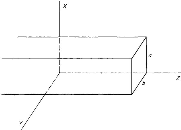
FIG. 33.5. The rectangular waveguide.
