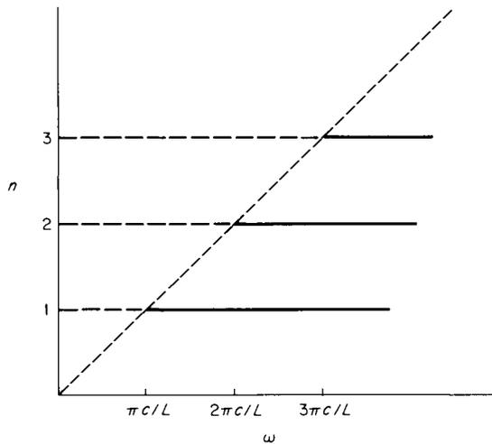
FIG. 33.3. Modes of propagation between two mirrors.
